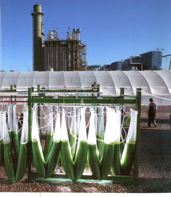
High hopes hang on bags of algae outside the Redhawk power plant near Phoenix. Researchers say the fast-growing green scum, fed by power plant exhaust, could soak up carbon dioxide while cranking out 5,000 gallons of biodiesel an acre each year—at least in theory. □
