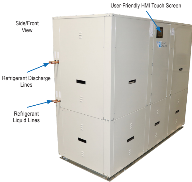
OC Refrigerant Connections: Discharge Line- 7/8" (2), Liquid Line- 5/8" (2)
