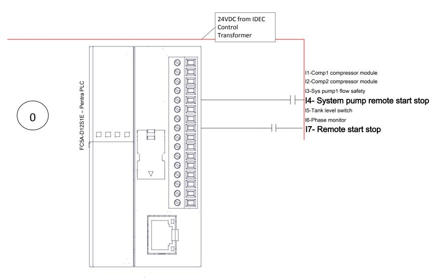
Remote start stop feature, field installation notes: Both remote chiller and system pump start stop are field installed features. Once installed, these features must be enabled via the factory configuration section of the chillers HMI touchscreen. Please contact Legacy Technical Support for instruction on access to Factory configuration section of your chillers HMI touchscreen.
