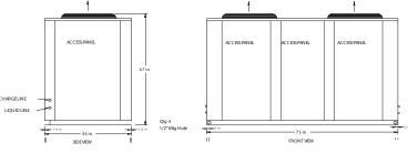
OC Refrigerant Connections: Discharge Line- 3/4" (2), Liquid Line- 1/2" (2)
